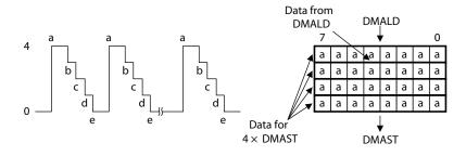
In Figure 16–27, each DMALD requires four entries and each DMAST removes one entry.
