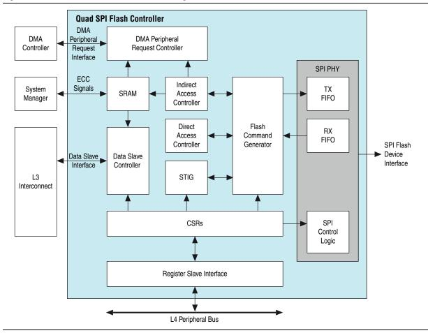
The quad SPI controller consists of the following blocks and interfaces:
