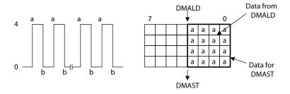
Each DMALD in the program loads two 64-bit data transfers into the MFIFO buffer. Because the destination address is a 32-bit fixed address then the DMAC splits each 64-bit data item across two entries in the MFIFO buffer.
