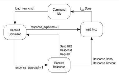
The command path state machine performs the following functions, according to cmd register bit values:
