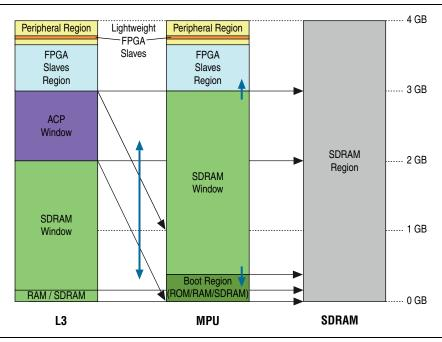
The window regions provide access to other address spaces. The thin black arrows indicate which address space is accessed by a window region (arrows point to accessed address space). For example, accesses to the ACP window in the L3 address space map to a 1 GB region of the MPU address space.
