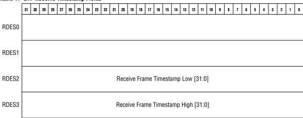
Table 17–22 on page 17–47 and Table 17–23 on page 17–47 describe the fields that have different meaning for RDES2 and RDES3 when the receive descriptor is closed and timestamping is enabled.
