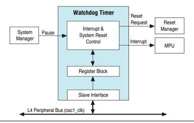
Each watchdog timer consists of a slave interface for control and status register (CSR) access, a register block, and a 32-bit down counter that operates on the slave interface clock (osc1\_clk). A pause input, driven by the system manager, optionally pauses the counter when a CPU is being debugged.
