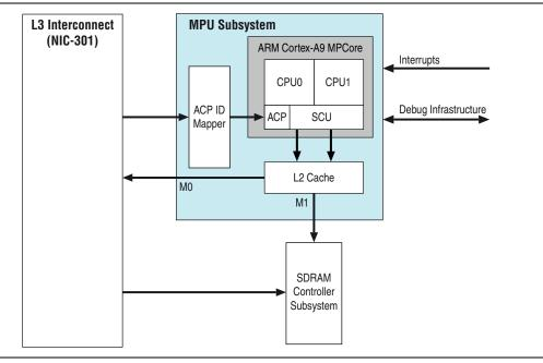
Figure 6–2 shows a block diagram of the Altera Cortex-A9 MPU subsystem.
