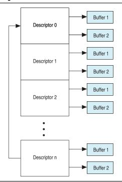
Figure 17-6. Descriptor Chain Structure
