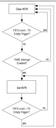
The threshold level is programmed into IIR\_FCR.TET. The available empty thresholds are empty, 2, ¼, and ½. The optimum threshold value depends on the system's ability to begin a new transmission sequence in a timely manner. However, one of these thresholds should prove optimum in increasing system performance by preventing the transmit FIFO buffer from running empty.
