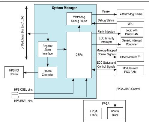
Figure 14-1. System Manager Block Diagram
