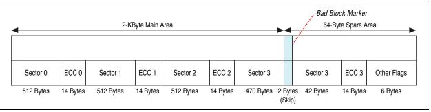
For detailed information about configuring the NAND flash controller for default, spare, or main+spare area transfer mode, refer to "Transfer Mode Operations" on page 10–25.
