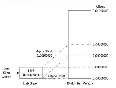
To remap the data slave to access other 1 MB regions of the flash device, enable address remapping in the enable AHB address remapping field (enabbremap) of the cfg register. All incoming data slave accesses remap to the offset specified in the remap address register (remapaddr).
