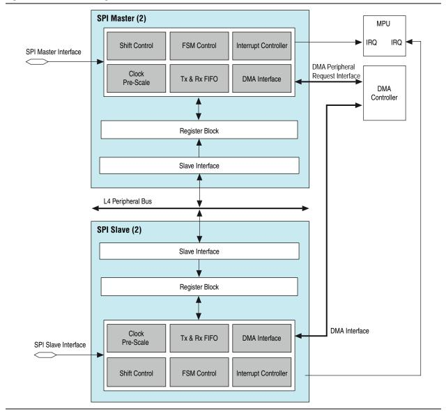
The functional groupings of the main interfaces to the SPI block are as follows: †
