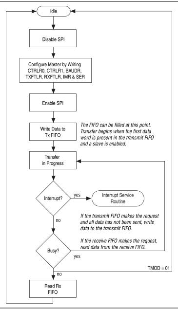
To complete an SPI or SSP serial transfer from the SPI master, follow these steps:
