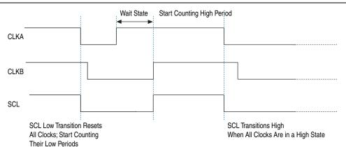
Figure 20–10. Multiple Master Clock Synchronization †
