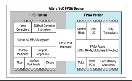
The HPS contains a microprocessor unit (MPU) subsystem with single or dual ARM® Cortex<sup>TM</sup>-A9 MPCore processors, flash memory controllers, an SDRAM controller subsystem, on-chip memories, support peripherals, interface peripherals, debug capabilities, and PLLs. The dual-processor HPS supports symmetric (SMP) and asymmetric (AMP) multiprocessing.
