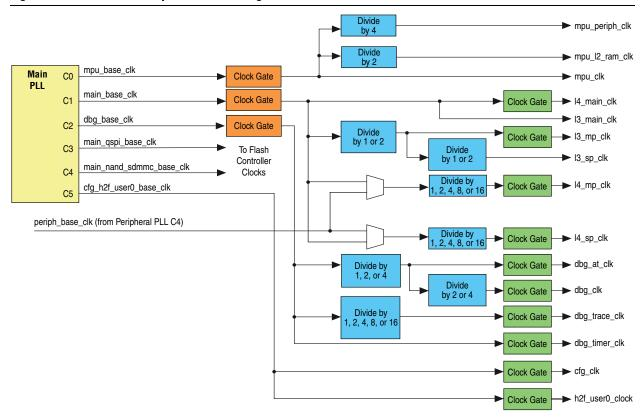
The clocks derived from main PLL C0-C2 outputs are hardware-managed, meaning hardware ensures that a clean transition occurs, and can have the following control values changed dynamically by software write accesses to the control registers:
