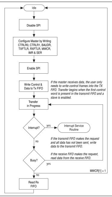
To complete a Microwire serial transfer from the SPI master, follow these steps:
