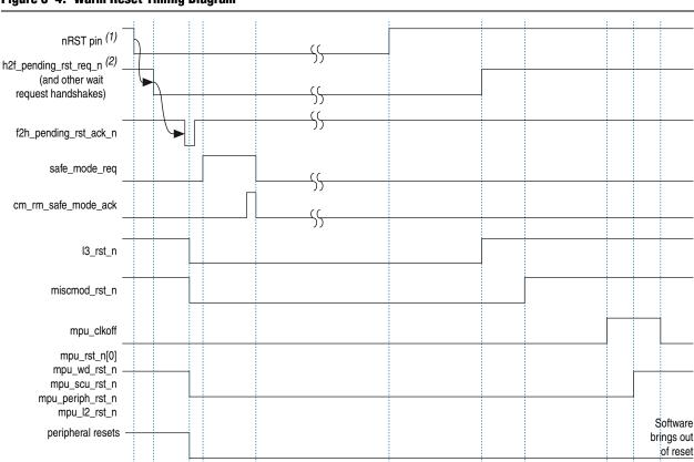
Figure 3–4 shows the timing diagram for warm reset.
