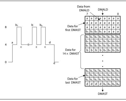
The DMALD shown as **d** does not increase the MFIFO buffer usage because it loads four bytes into an MFIFO buffer entry that the DMAC has already allocated to this channel.
