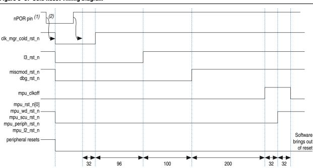
Figure 3-3. Cold Reset Timing Diagram
