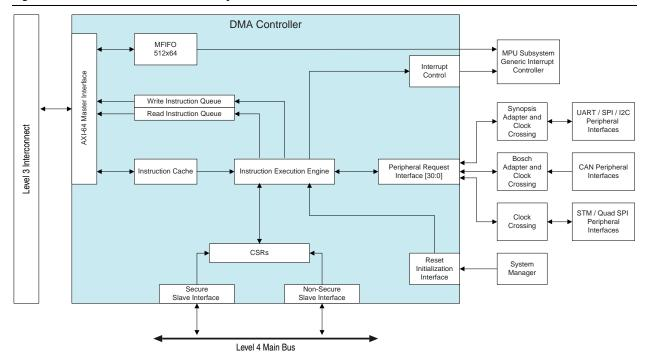
The DMA controller is driven by the 14\_main\_clk clock, which is used for the controller logic as well as all the interfaces. The DMA controller accesses the level 3 (L3) main switch with its 64-bit AXI master interface.
