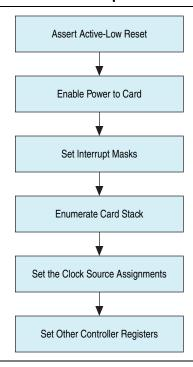
Software must perform the following steps after the power-on-reset:
