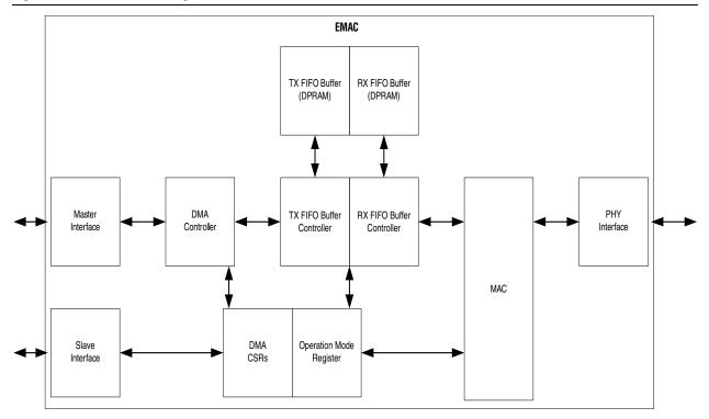
There are two host interfaces to the MAC. The management host interface, a 32-bit slave interface, provides access to the CSR set. The data interface is a 32-bit interface. It controls data transfer between the direct memory access (DMA) controller channels and the rest of the HPS system through the NIC-301 L3 interconnect.
