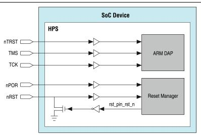
The test reset (nTRST), test mode select (TMS), and test clock (TCK) pins are associated with the TAP reset domain and are used to reset the TAP controller in the DAP. These pins are not connected to the reset manager.
