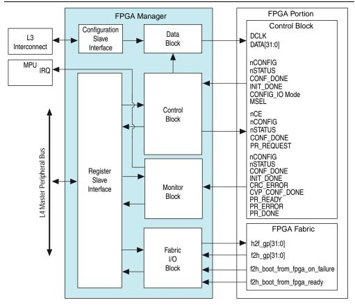
The register slave interface connects to the level 4 (L4) master peripheral bus for control and status register (CSR) access. The configuration slave interface connects to the level 3 (L3) interconnect for the microprocessor unit (MPU) subsystem or other masters to write the FPGA configuration image to the FPGA control block (CB) when configuring the FPGA portion of the SoC device.
