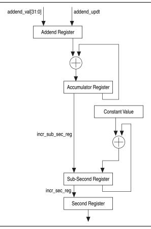
The System Time Update logic requires a 50-MHz clock frequency to achieve 20-ns accuracy. The frequency division ratio (FreqDivisionRatio) is the ratio of the reference clock frequency to the required clock frequency. Hence, if the reference clock ( $clk_ptp_ref_i$ ) is, for example, 66 MHz, this ratio is calculated as 66 MHz / 50 MHz = 1.32. Hence, the default addend value to be set in the register is 232 / 1.32, 0xC1F07C1F.
