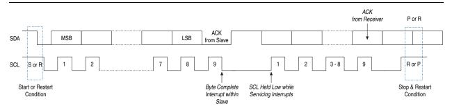
Figure 20-2. Data transfer on the I<sup>2</sup>C Bus †
