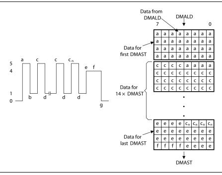
The DMALD shown as **f** does not increase the MFIFO buffer usage because it loads four bytes into an MFIFO buffer entry that the DMAC has already allocated to this channel.
