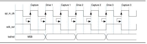
The frequency of sclk\_out can be derived from Equation 19–1, where <*SPI clock*> is spi\_m\_clk for the master SPI modules and 14\_main\_clk for the slave SPI modules. †
