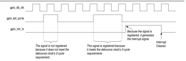
Enabling the debounce circuitry increases interrupt latency by two clock cycles of the debounce clock.
