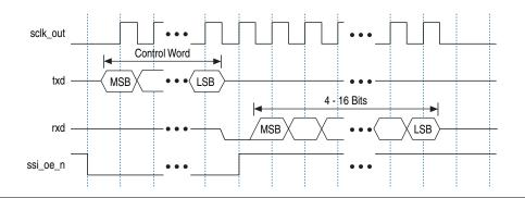
Figure 19–10 shows the timing diagram for a single SPI serial slave write to an external serial master.
