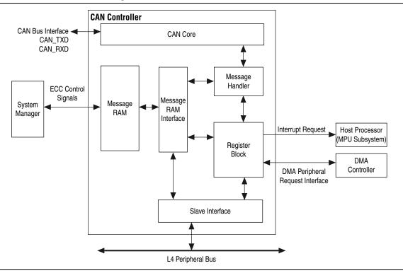
The CAN controller consists of the following modules and interfaces:
