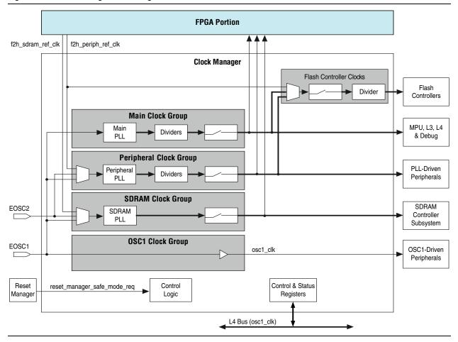
The next section describes the functional blocks internal to the clock manager. Refer to Figure 2–3 to Figure 2–6 for more detailed versions of the grey boxes in Figure 2–1.
