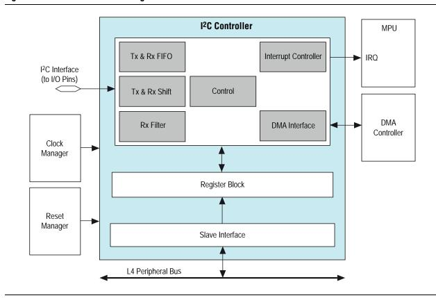
The I<sup>2</sup>C controller consists of the following modules and interfaces:
