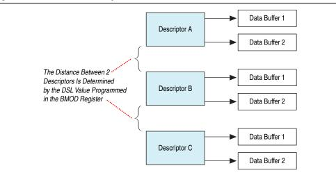
Figure 11-5. Chain Descriptor Structure
