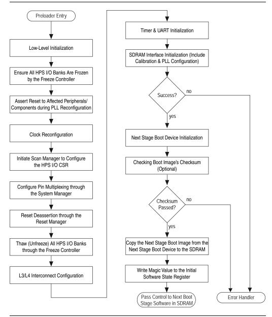
Low-level initialization steps include reconfiguring or disabling the L4 watchdog 0 timer, invalidating the instruction cache and branch predictor, remapping the on-chip RAM to the lowest memory region, and setting up the data area.
