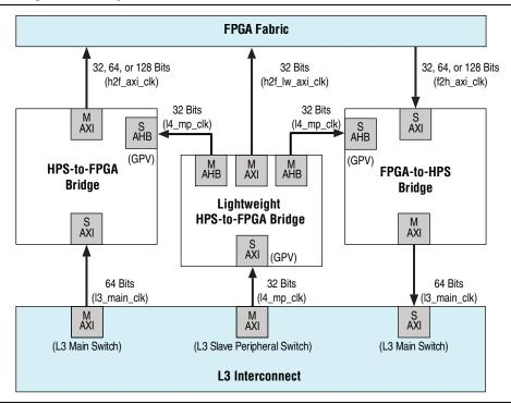
The HPS-to-FPGA bridge is mastered by the level 3 (L3) main switch and the lightweight HPS-to-FPGA bridge is mastered by the L3 slave peripheral switch.
