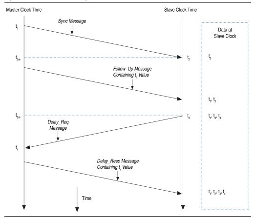
Figure 17-3. Networked Time Synchronization
