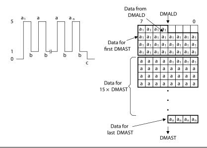
The first DMALD instruction loads four doublewords but because the destination address is unaligned, the DMAC shifts them by four bytes and therefore it uses five entries in the MFIFO buffer.
