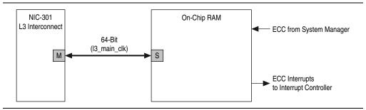
Transfers between memory and the NIC-301 L3 interconnect happen through a 64-bit interface, gated by the 13\_main\_clk interconnect clock. ECC logic detects single-bit, corrected and double-bit, uncorrected errors. The memory has a read acceptance of two, a write acceptance of two, and a total acceptance of two with round-robin arbitration.
