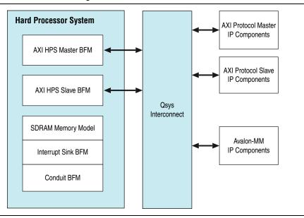
The HPS BFMs use standard function calls from the Altera® BFM application programming interface (API), as detailed in the remainder of this section.
