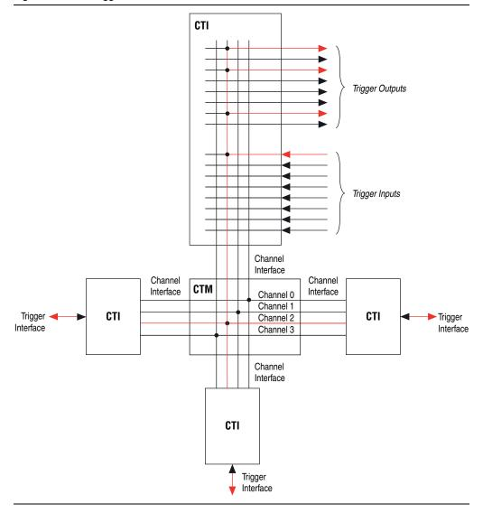
Figure 7–5. CTI Trigger Connections
