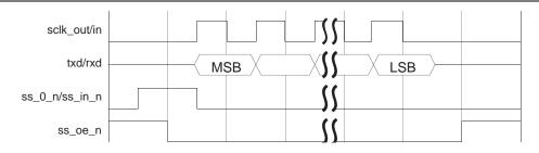
Continuous data frames are transferred in the same way as single data frames. The frame indicator is asserted for one clock period during the same cycle as the LSB from the current transfer, indicating that another data frame follows. Figure 19–8 shows the timing for a continuous SSP transfer. †
