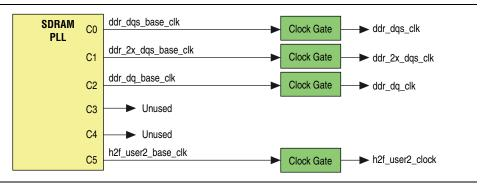
The SDRAM PLL output clocks can be phase shifted in real time in increments of 1/8 the VCO frequency. Maximum number of phase shift increments is 4096.
