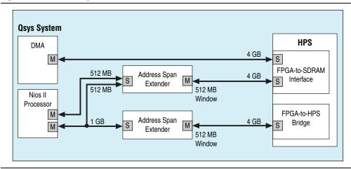
You can also use the address span extender in the HPS-to-FPGA direction, for slave interfaces in the FPGA. In this case, the HPS-to-FPGA bridge exposes a limited, variable address space in the FPGA, which can be paged in using the address span extender.
