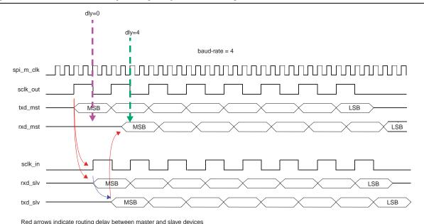
Blue arrow indicates sampling delay within slave from receiving slk\_in to driving txd out
