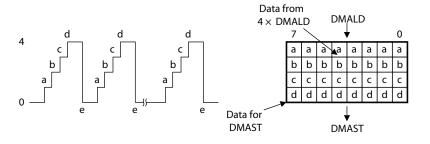
In Figure 16–26, each DMALD requires one entry and each DMAST removes four entries.
