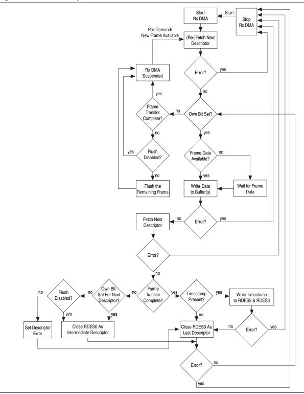
If software has enabled timestamping through CSR, when a valid timestamp value is not available for the frame (for example, because the receive FIFO buffer was full before the timestamp could be written to it), the DMA writes all-ones to RDES2 and RDES3. Otherwise (that is, if timestamping is not enabled), the RDES2 and RDES3 remain unchanged. †
