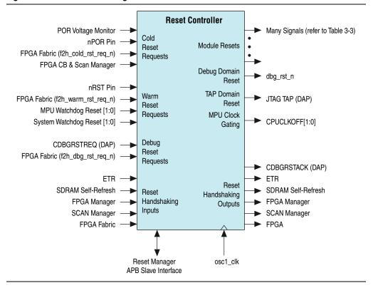
The reset controller supports the following cold reset requests:
