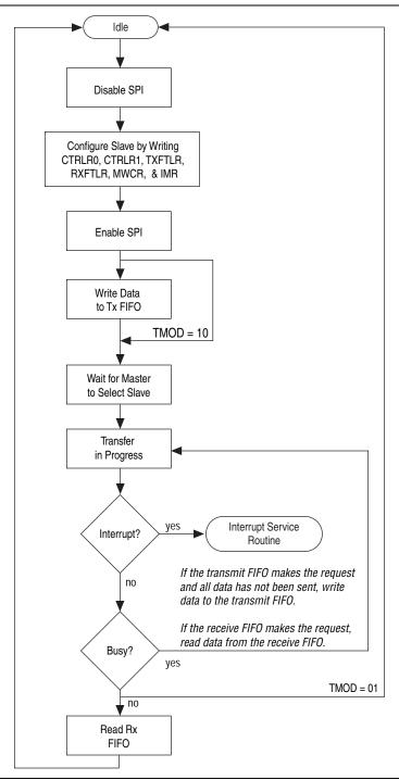
To complete a continuous serial transfer from a serial master to the SPI slave, follow these steps:
