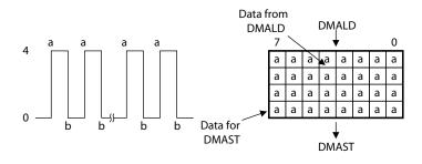
In Figure 16–25, each DMALD requires four entries and each DMAST removes four entries.
