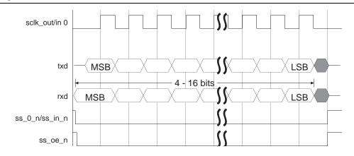
There are four possible transfer modes on the SPI controller for performing SPI serial transactions; refer to "Transfer Modes" on page 19–7. For *transmit and receive transfers* (transfer mode field (9:8) of the Control Register 0 = 0), data transmitted from the SPI controller to the external serial device is written into the transmit FIFO buffer. Data received from the external serial device into the SPI controller is pushed into the receive FIFO buffer.  $\dagger$
